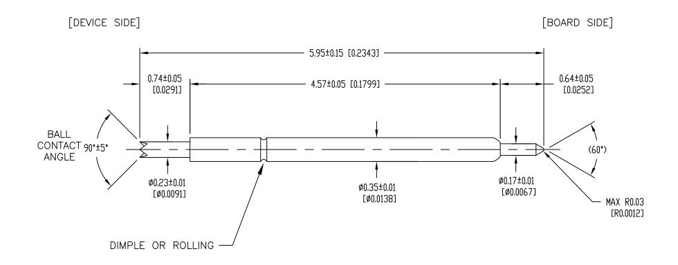
It is very important to verify actual working travel when this probe is set in a socket due to difference of only 0.13mm between recommended and full travel. In case that the actual working travel is over 0.51mm, the device, spring, plunger and/or PCB pad will be damaged. Therefore, the above notice must be reflected in socket design.
